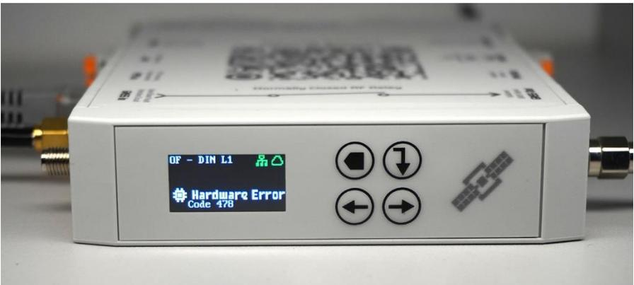
Once the GNSS antenna is connected, this error will be resolved. The probe will show the status "Connecting" and then "Offline":
